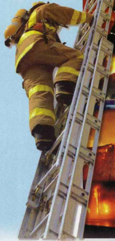
Three Fold Trussed Ladder
